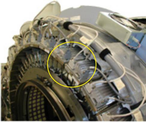
**Figure 8:** Distributed digitization units. Example digitizer circled in yellow.
