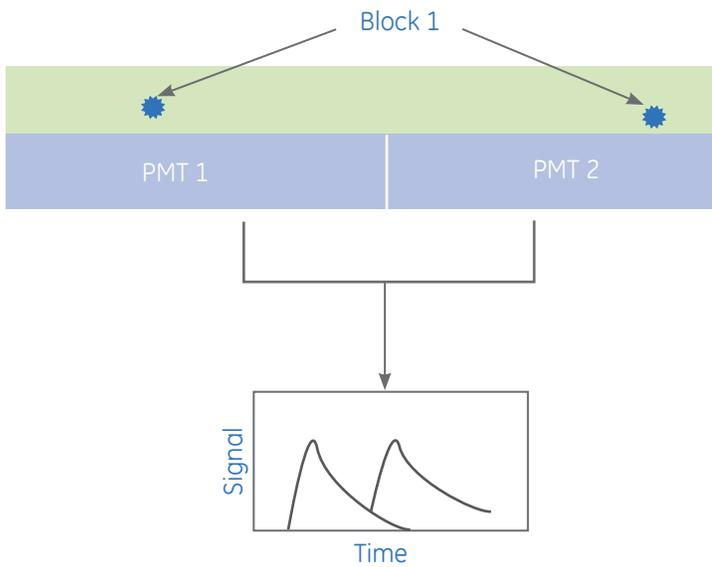
**Figure 5:** Pile up in single detector that covers a large surface area
