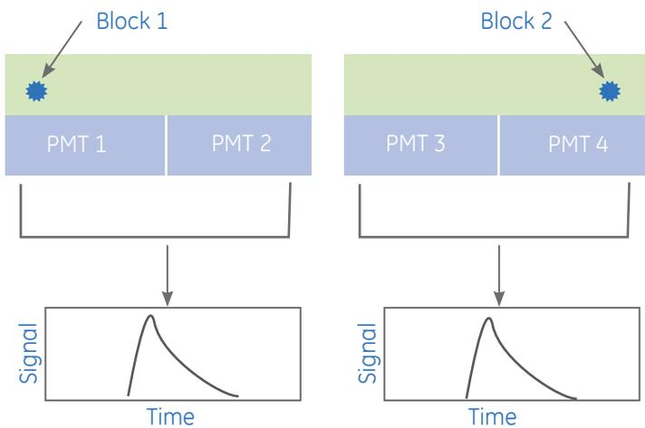
**Figure 6:** Reduced signal pileup with two smaller blocks that cover the same surface area as the single block shown in figure 5.
