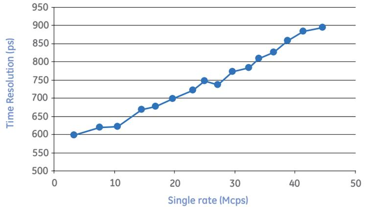
**Figure 7:** Temporal resolution vs countrate for a competitor's large area detector (Surti et al., JNM 2007)
