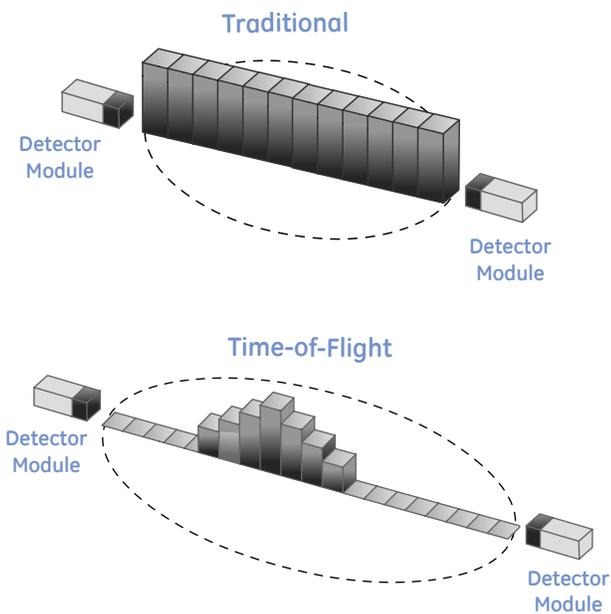
**Figure 3:** Traditional and TOF projection examples.
