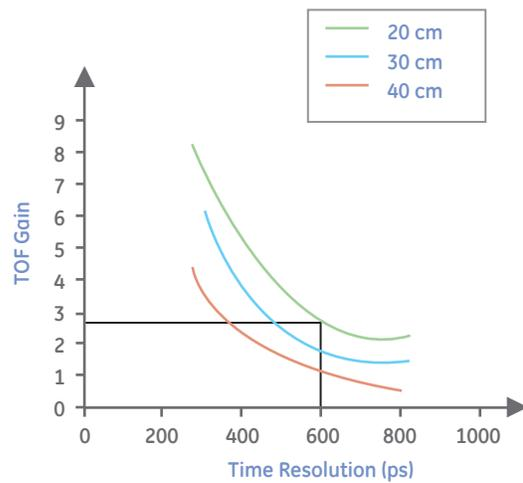
**Figure 4:** Plot of estimated TOF gain as a function of uniform activity diameter and timing resolutions.
