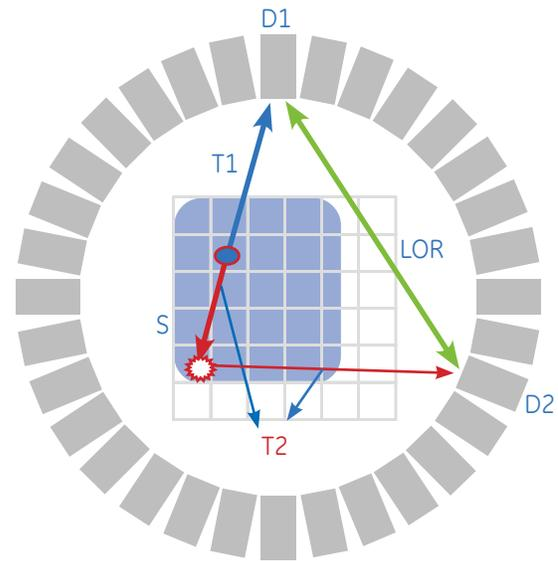
**Figure 9:** Conversion of flight distance into time difference for TOF scatter correction.
